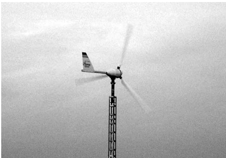
Figure 10 A 12-kW wind turbine at the CEDER test plant.
