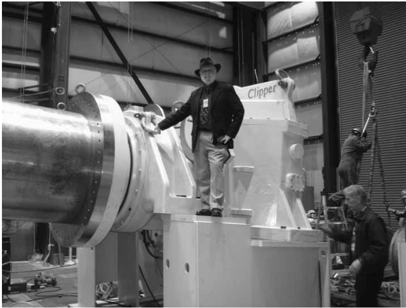
Figure 6 Robert Thresher, director of the National Wind Technology Center at NREL, and the Clipper Windpower 2.5-MW drivetrain at the facility's dynamometer test stand.
