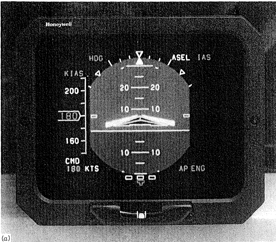
Figure 9.1 Electronic displays (a) Vertical Situation Display (VSI), courtesy of Honeywell; (b) Horizontal Situation Display (HSI), courtesy of Smiths Industries Aerospace.
