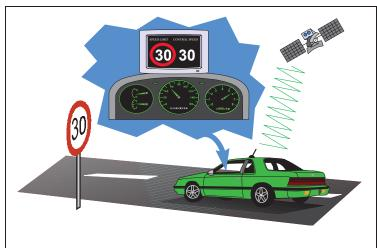
Figure 1: Concept of autonomous ISA system
