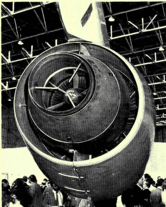
Left The BAe 146 is powered by four ALF502s slung in underwing pods. The aircraft's wings are made by Avco's Aerostructures division
