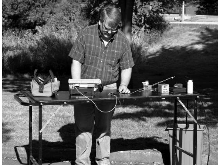
Figure 15.14. A fiber-optic worktable used for acceptance testing. [Credit: The Light Brigade.]
