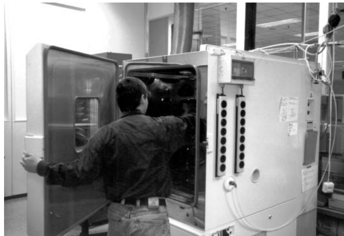
Figure 15.2. Temperature chamber for testing OTDRs. [Credit: The Light Brigade.]
