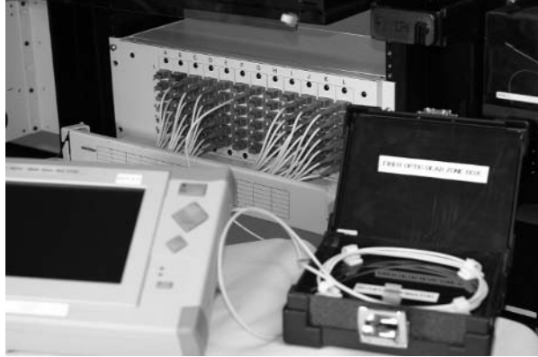
Figure 3.3. Typical mini-OTDR linked to a fiber-optic patch panel. [Credit: The Light Brigade.]
