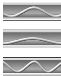
Figure 5.9. Optical fiber inside a loose buffer tube. [Credit: The Light Brigade.]
