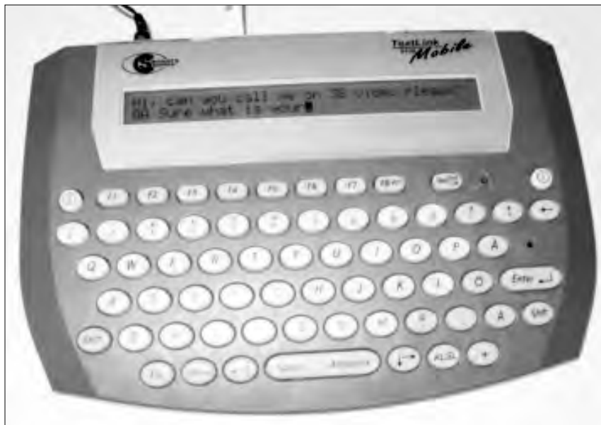
Figure 17.7 Legacy text phone for use on the PSTN
